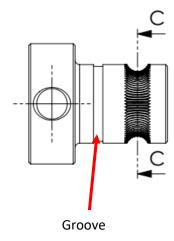
NEW: Pro drive wheel, without groove check for the **PD** or **pro drive** in the name
