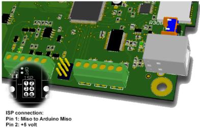
Pin 2: +5 volt Pin 3: SCK to Arduino SCK Pin 4: MOSI to Arduino MOSI Pin5: Reset to Arduino pin 10 (ss) Pin 6: GND to Arduino GND
