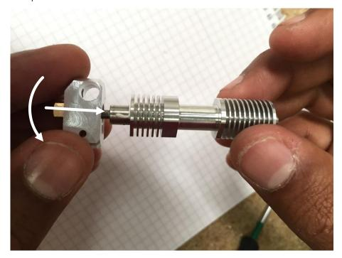
Ensure the hot-end parts are kept together. This can be done by compressing the ends by hand, but a clamp will also do the job.
