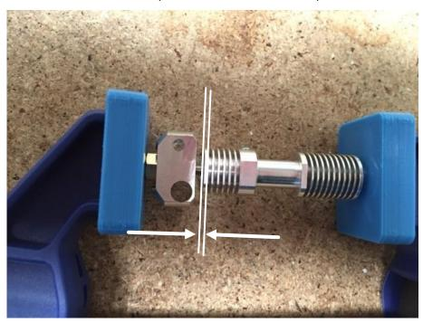
Fix the Set screw D-916 - M3 x 4 as tight as possible, without damaging the threads.
