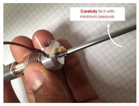
Take the heater for extruder (ID8). Push the heater till the end of the barrel. Ensure it doesn't stick out. The heater is not so vulnerable as the thermistor and can be fixed firmly.
