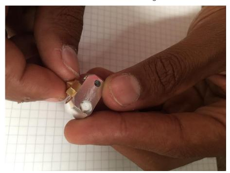
Take Heatbreak (ID3) and turn it into the barrel until it loosely touches the nozzle.
