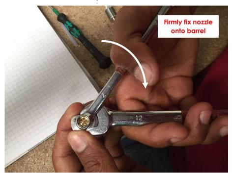
Double check if the nozzle is fixed against the heat-break and NOT the heater barrel. This can be confimed by checking if there is a tiny gap between the nozzle flange and the heater barrel.
