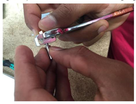
Take wrench 12 and 7mm and fix the nozzle firmly onto the heat-break.
