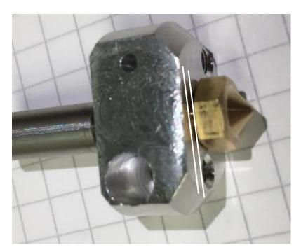
Place the teflon tube in the heat-break. Take some cooling paste and apply it on the top part of the heat break. This step is essential to provide proper heat transfer from heat break to hot-end base.
