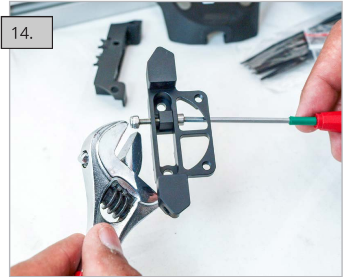
14. Assembly of NEW mover and bracket including M3 x 20 bolt.
