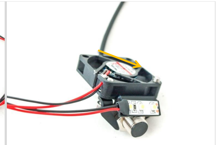
106 Remove adhesive backing of the LED strip. Place LED-strip onto the bracket.
