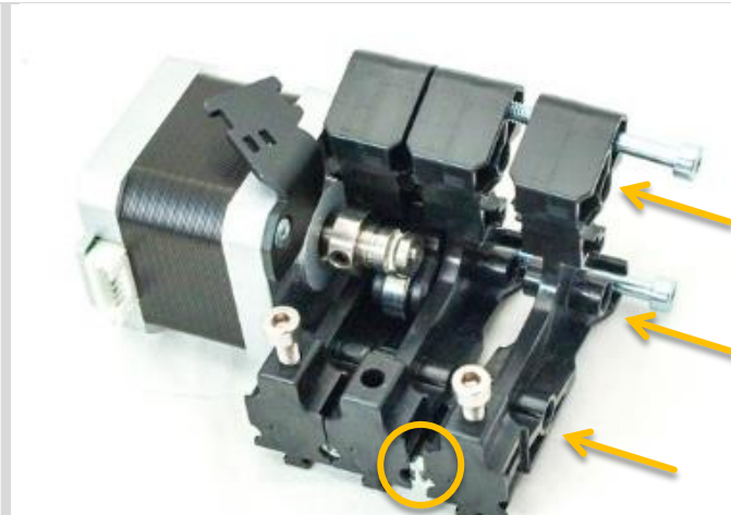
80 (1x) Plastic part Slide part onto the assembly. Make sure the square nut is placed correctly. Tools
