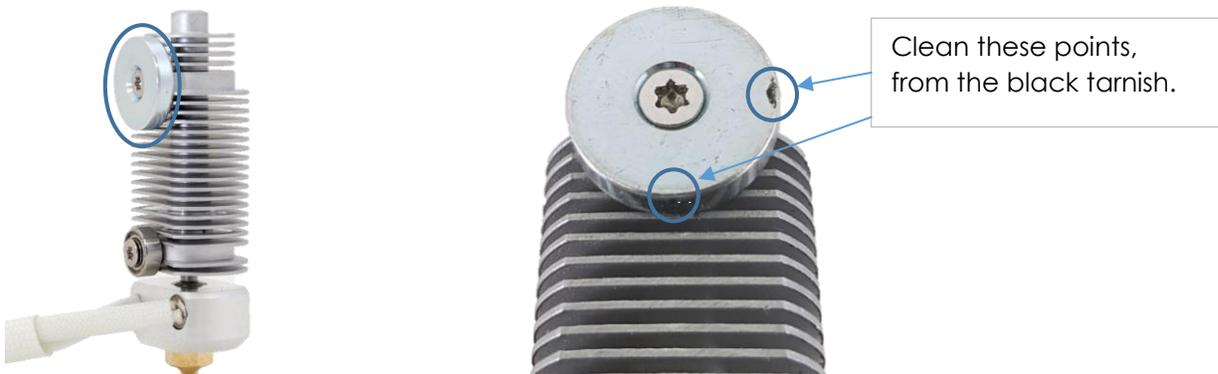
**RECOMMENDED:** Put non-electrically conducting teflon spray on the disc. This improves the probe working and also improves the electrical contact for the long term.
