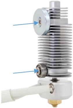
Note: Also the bearing on the bottom should be properly fastened. This does not prevent z-sensor triggered message, but ensures proper operation of the printer.
