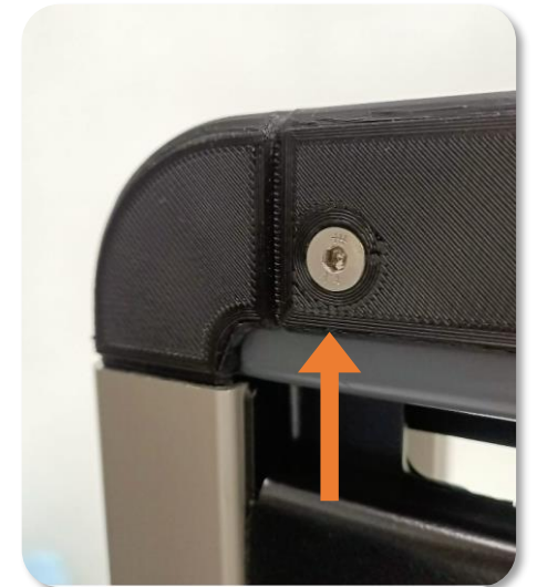
Remove the two inbus bolts (inbus size 3mm)
