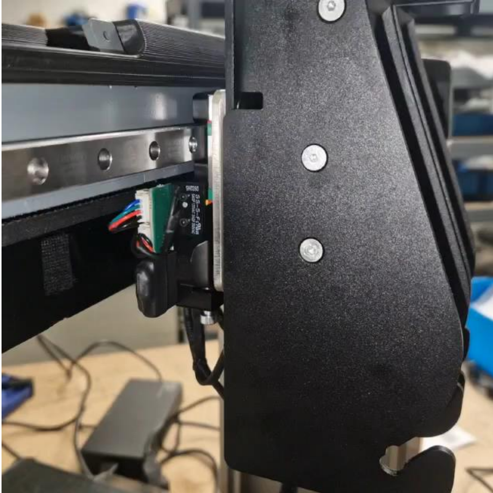
Compensation is adjusted and the z-probing movement goes smoothly again
