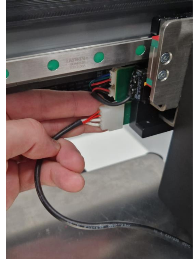
12. Slide the connector over the PCB. (see cable configuration)
