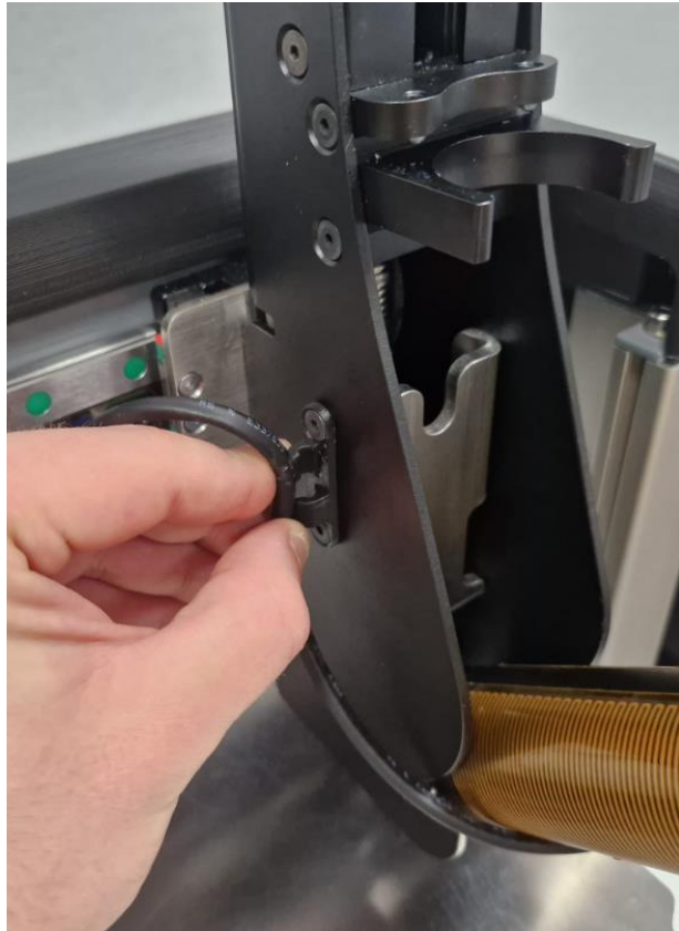
14. Place the cable in the cable clamp at the left side of the extruder.
