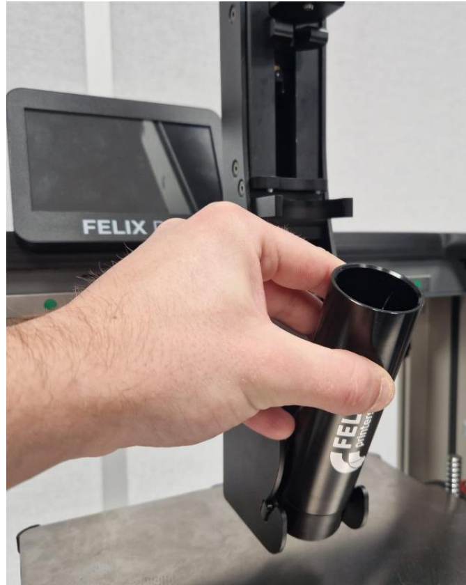
2. Remove the old tube/syringe holder.
