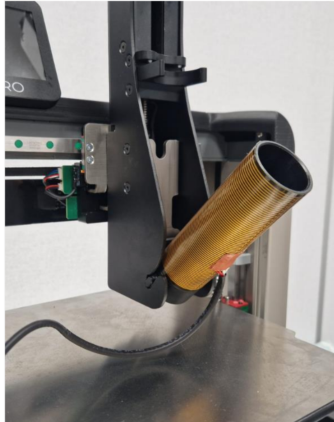
11. Place the heated tube in the extruder.
