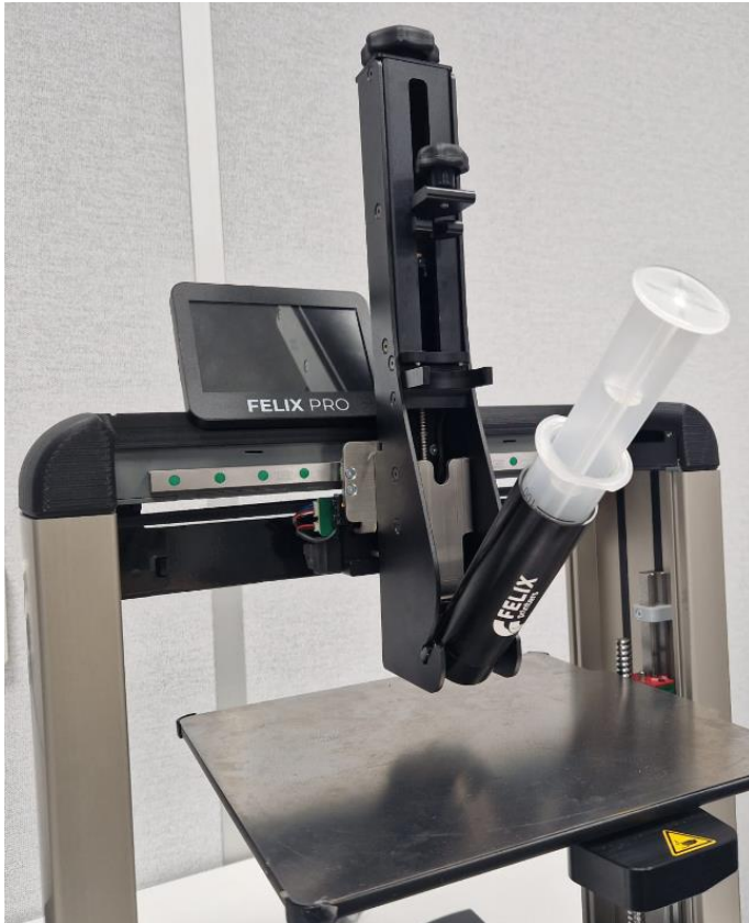
1. Remove the syringe if there is one loaded in the machine.
